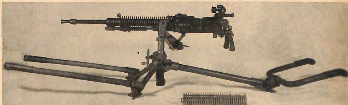
Figure 182. Model 92 (1932) 7.7-mm heavy machine gun—showing carrying handles and ammunition strip.
